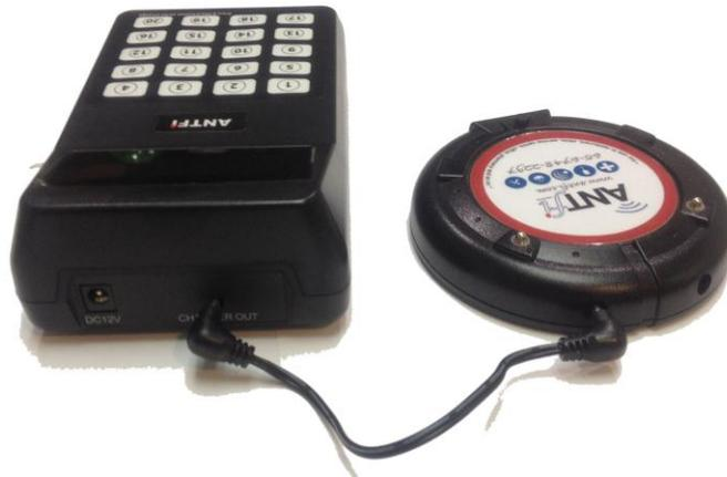
2. Next plug the round power connector of the power adapter into the classic transmitter jack **1** as shown below.
