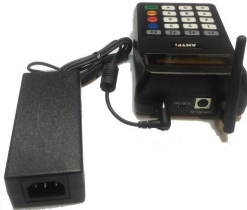
2. Next plug the power adapter into the power cable, and then plug the power cable 3-pin connector to the wall power source.
